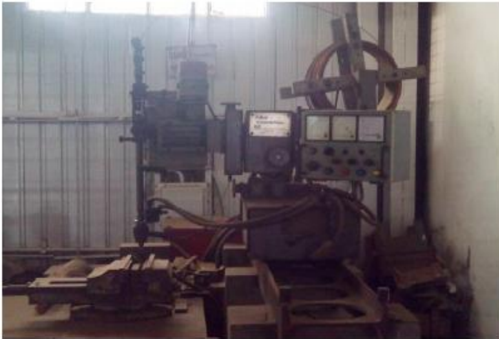
Fig 3: Photographic view of the set up of Submerged arc welding
